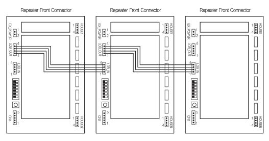
■ Wiring Diagram between a Repeater and a Wall Pad
